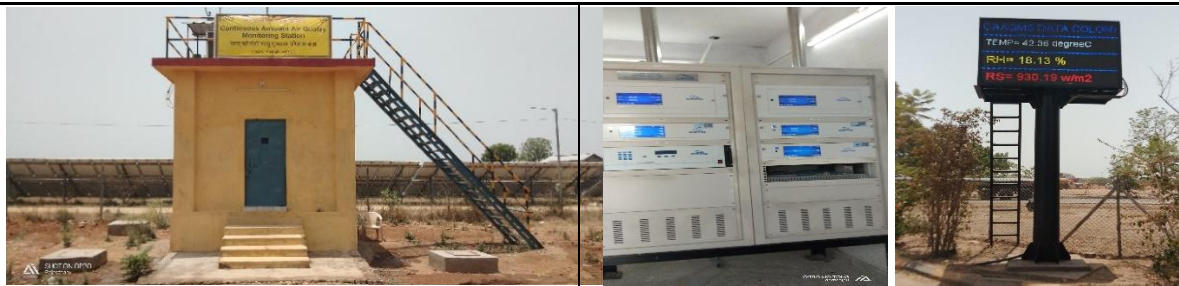
Visuals of CAAQMS, Analyzers and display Board
