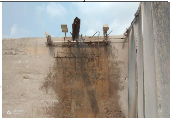
Water Sprinkling system at Crusher hopper
