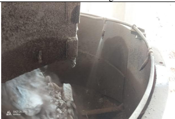
Water fogging System arrangement at Cone Crusher
