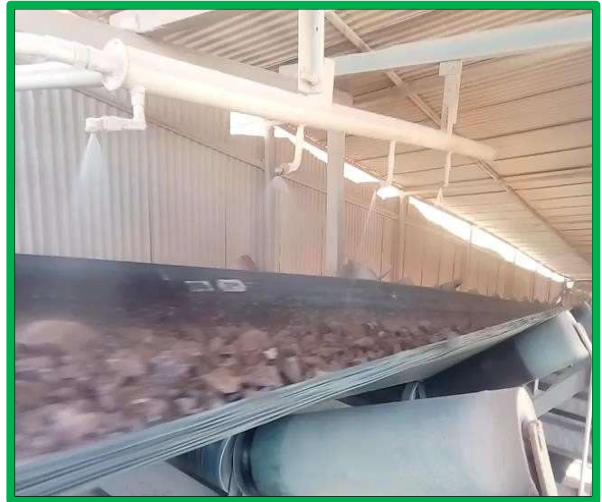
As a dust control measures we have installed Bag houses and Water sprinkling system over conveyor belts.
