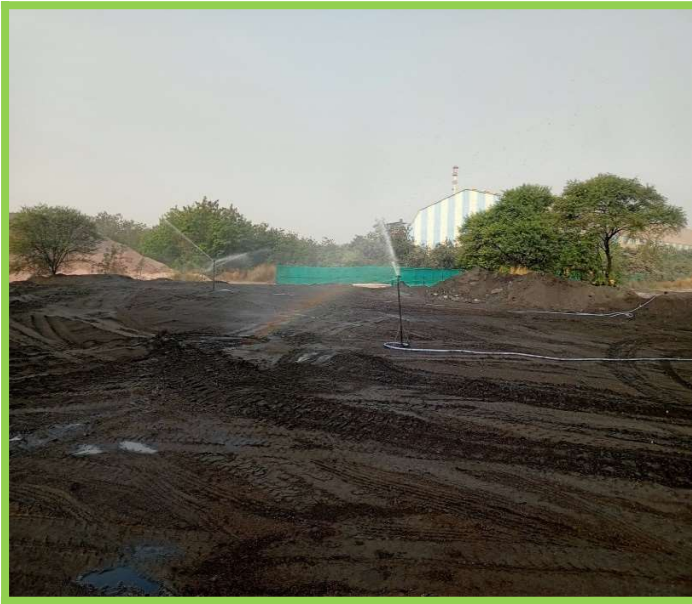
Water sprinklers all around the coal stockpiles to control fugitive dust emission.
