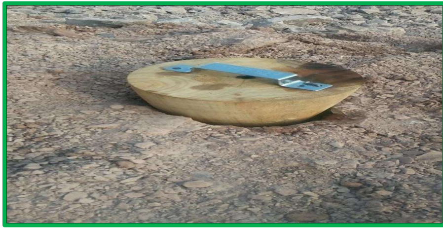
After drilling all drill holes are being plugged with wooden collar cones.
